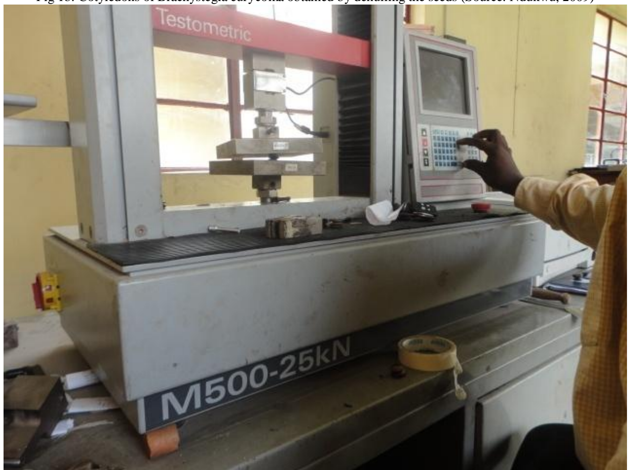
Figure 2: Universal Testing Machine with Brachystegia Eurycoma seeds loaded in the lateral Orientation
