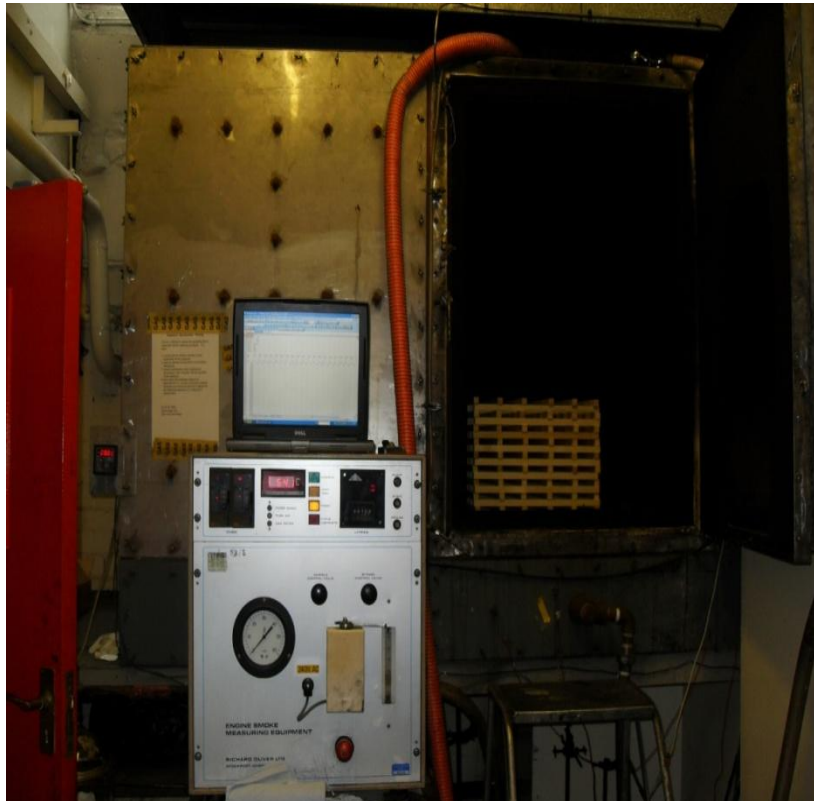
Figure 1: Photograph showing the fire rig enclosure with wood crib inside
